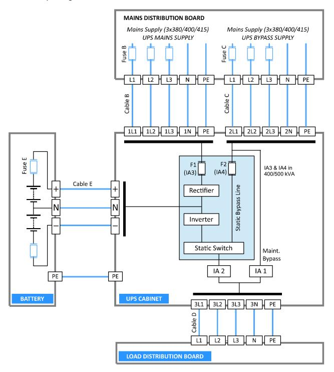
Note: The input and bypass supply neutrals are connected to a common neutral busbar
