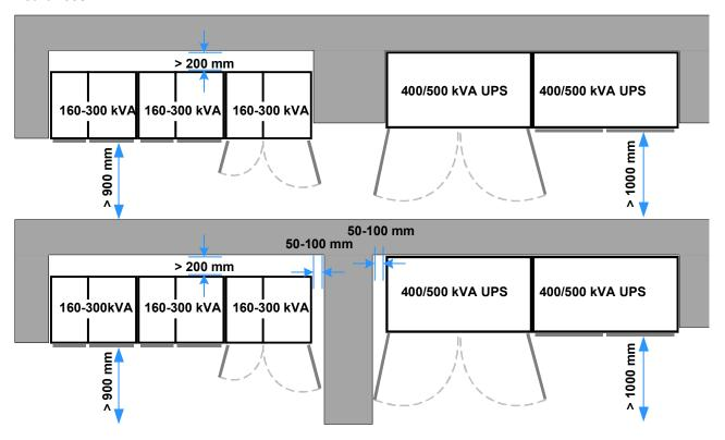
The above diagram illustrates the recommended clearances to be provided around the UPS cabinets.
