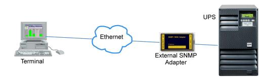
The external SNMP adapter is enclosed in a small box which must be powered from a backed-up supply supported by the UPS output so that its power is maintained in the event of a mains failure. A suitable plug-top power supply is included with the option kit.
